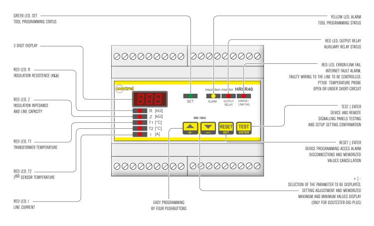
Wherever it is necessary to guarantee safety and operational continuity and prevent power supply interruptions, such as hospitals and other medical locations, insulation transformers and devices detecting and signalling any first fault to earth have to be used. Risks arising from the use of a traditional insulation monitor:
